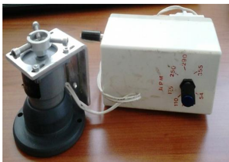
Photo 1. Home-made rotating apparatus for minimizing the under-sampling problems
