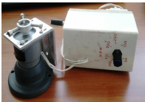
Fig 1b. Home-made rotating apparatus for minimizing the under-sampling problems
